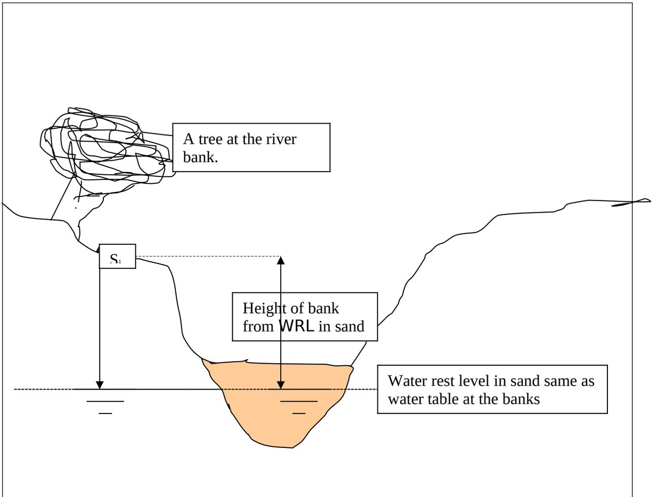
*This figure explains the relationship between the water levels in the river channel and at the banks. Table 1 confirms this hypothesis.*
